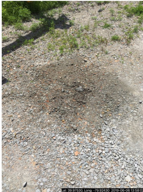
Photo # 8. Staining on the pad gravel on the southern edge of the pad.
