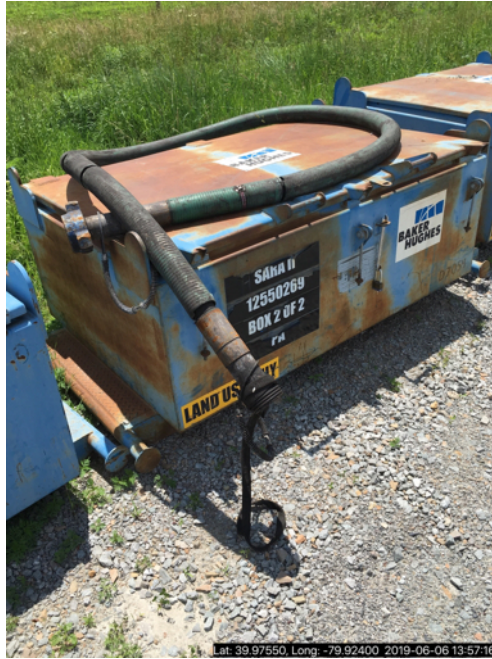
Photo # 7. A contaminated hose stored off containment on the southern side of the pad.
