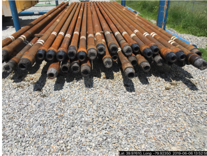
Photo # 3. An equipment rack found without containment, note multiple small stains under rack.
