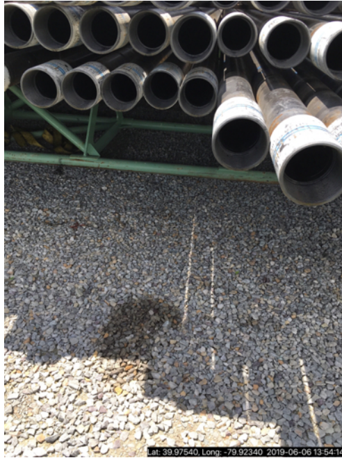
Photo # 5. A second equipment rack found without containment, note staining under equipment.
