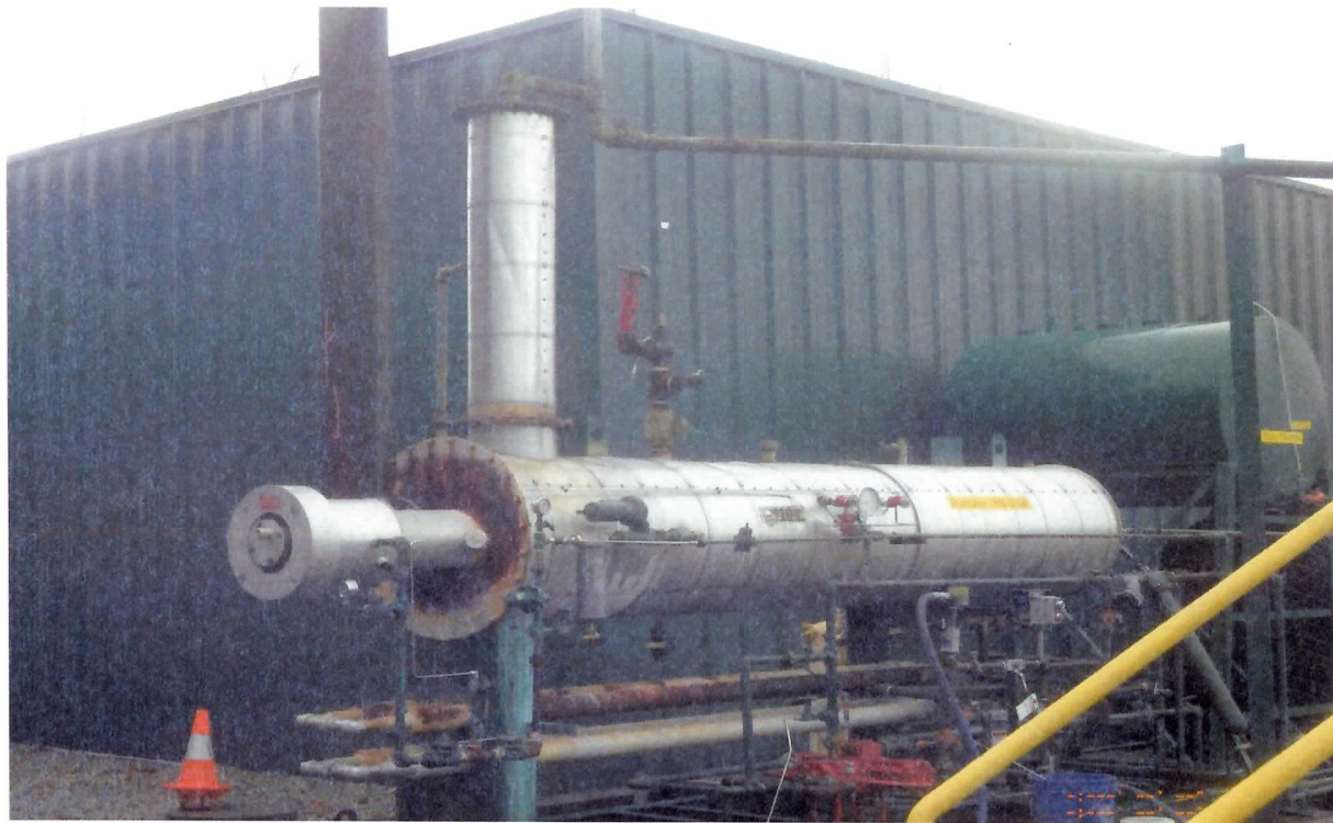
4. 25MMscf/day dehydrator reboiler – LMM Springhill CS – 11/10/2015
